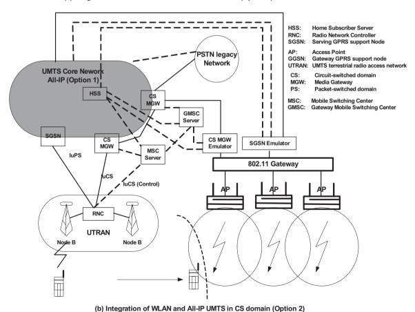
Fig. 4. Tightly coupled integration (simplified) of WLAN and all-IP UMTS: (a) *Option 1* in PS domain; (b) *Option 2* in CS domain.
