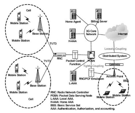
Fig. 2. Tightly-coupled and loosely-coupled in CDMA2000.
