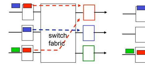
output port contention: only one red datagram can be transferred. lower red packet is blocked one packet time later: green packet experiences HOL blocking
