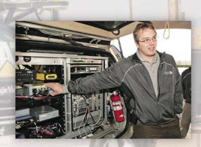
Chris Urmson, Director of Technology for Tartan Racing, shows the computers and electronics that are embedded in the Tartan Racing vehicle. The rear cargo area also includes a safety system that allows the vehicle to be stopped via a radio signal, if needed.
