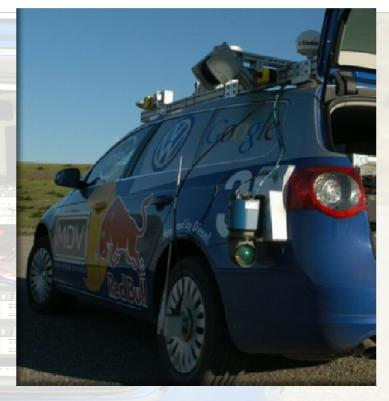
"The POS LV system generates precise, robust positioning and orientation information for mobile data acquisition systems. The system combines all the advantages of GPS with those of inertial technology, to provide continuous and accurate data. By utilizing the POS LV system, data capture can be undertaken quickly and efficiently."
