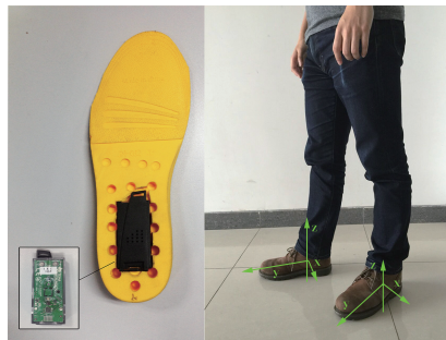
Fig. 1. The SensorTag used in FootStep-Tracker. We embed two tags into the insoles and use an Android phone to collect and process the sensor data.
